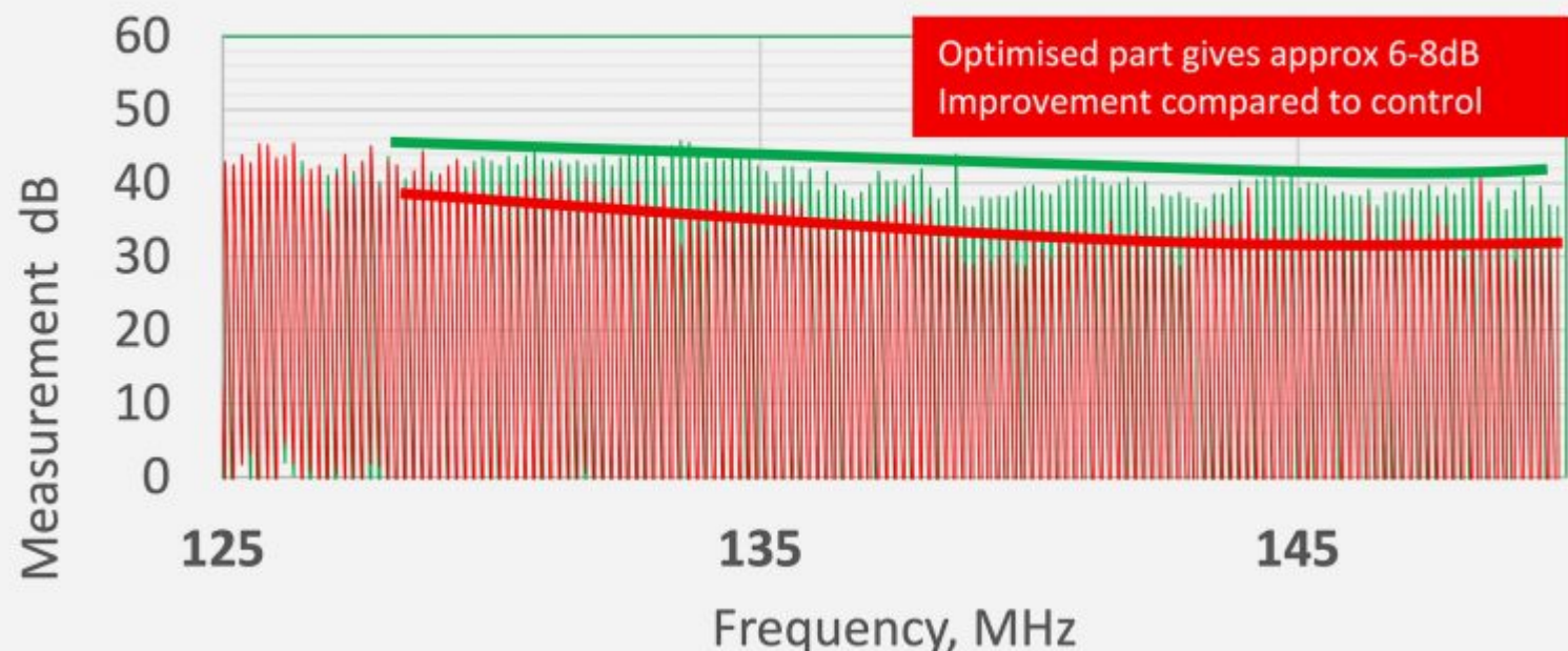
Fig. 1: Comparison of radiated emission on motor-drive board using close field probe
